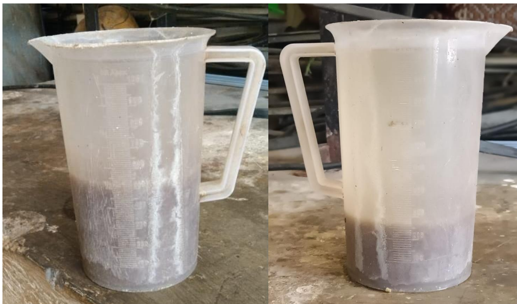
Figure 4: MLSS method used by STP Operator to check treated water batch quality.
