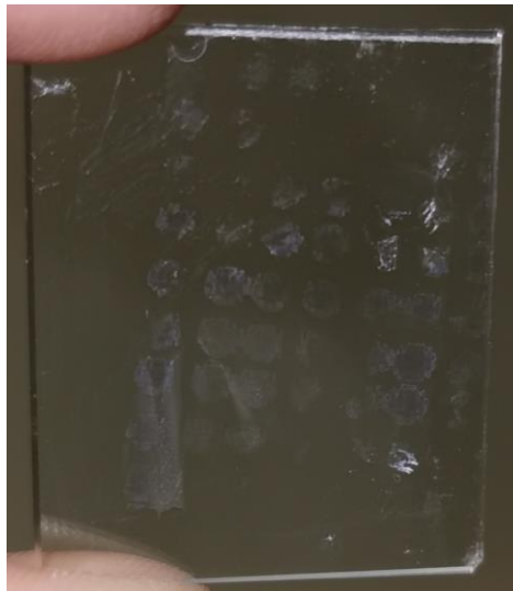
Figure 27: First successful pattern transfer via UV-Lithography with FTM coated AR-N-4400-05 on a microscope slide.
